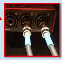
Input cables for the drum set. One plugs into Input 3 and the other into Input 4.
