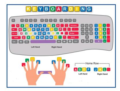
**QWERTY** keys were arranged diagonally on typewriters to provide space for the levers. This layout was kept for electronic keyboards. Each diagonal column has a dedicated finger.
