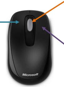
In the middle most mouses have a wheel, rolling the wheel backwards and forwards will cause websites to scroll up and down
