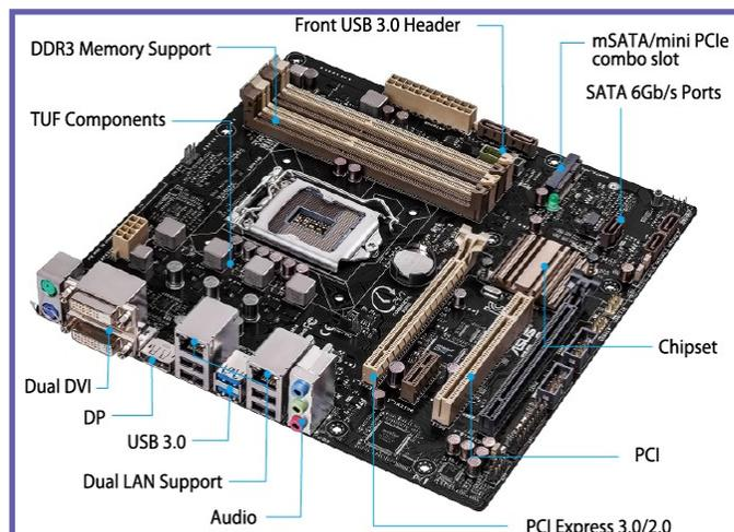
Before installing in the case, it is recommended to install the processor, cooling fan, and memory onto the motherboard while it is easily accessible. Take the motherboard out of the box and anti-static bag. Place the motherboard on a hard, flat, non-metal desk like a wood desk or the top of the motherboard box. Do not place the motherboard on top of the anti-static bag, since the outside can conduct electricity. Please read the instructions for any special component installations.
