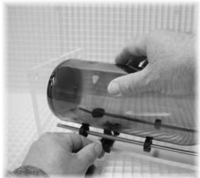
4. You will notice a small Black Line at the top, center, of the base piece. Make a mark on the bottle with a Sharpie Marker. This will be your starting point in line with the base mark. This way you will have a visual indication that you have rotated the bottle 360 degrees. **WARNING: Never rotate the bottle more than 360 degrees. Over-scoring will result in a bad break and diminished cutting wheel life.**
