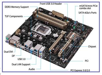
state drive compatible. Just like cases, motherboards come in micro ATX and ATX size (ATx being full size). Recommended brands are MSI or Asus, and price starts at \$65.
